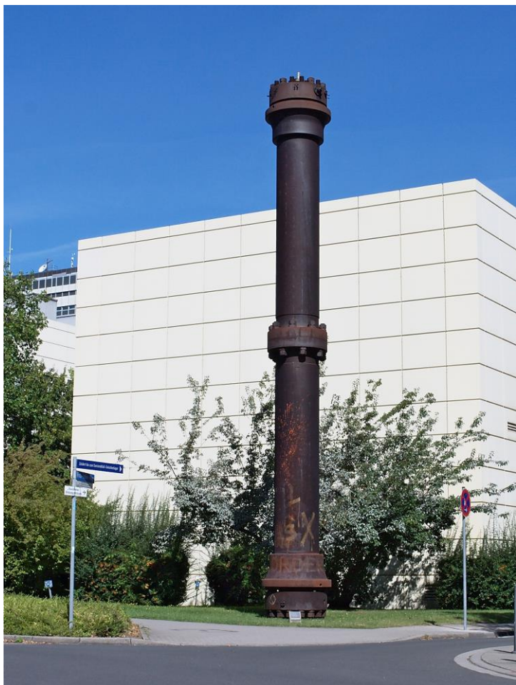
A historical (1921) high-pressure steel reactor for production of ammonia via the Haber process is displayed at the Karlsruhe Institute of Technology (KIT), Germany
